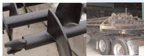
It has been observed that epoxy coating on the auger portion of the anchor can be significantly abraded during the installation process. However, and oftentimes, the epoxy coating remains intact and relatively undisturbed on the shaft portion of the anchor. Because only the upper portion of the exterior shaft near the surface needs protection, epoxy coating may actually be superior to galvanizing for protecting the anchor from corrosion on a long-term basis.
